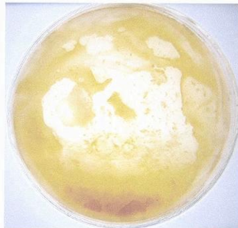
Fig. 3. Group 2 after 24 hr in darkness, showing bacterial growth on photocatalyst coating
