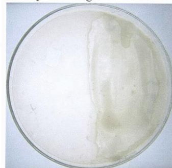
Fig. 4. No bacterial growth after 24 hr on photocatalyst coating (right side) under light illumination
